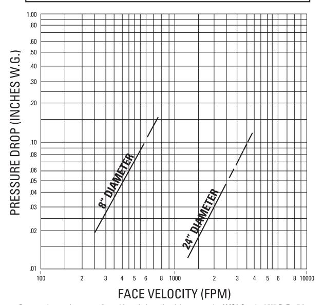
Pressure drop testing was performed by an independent laboratory to the AMCA Standard 500-D, Fig. 5.3 (ductwork upstream and downstream).
